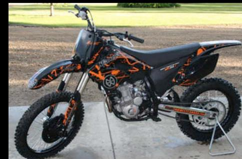
The Midwest NRG250-F is a radical contender with a dual overhead cam 249cc 4 stroke liquid cooled engine, electric start, 6-spd constant mesh transmission, cradled in a chromoly / aluminum frame, aluminum swing arm, no-link suspension, adjustable gas cell rear shock and 48 mm fully adjustable front forks smooth out trail or track.
