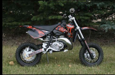
The Midwest NRG50 is all about performance, keeping the entry level racer in mind. We started with a 50cc 2 stroke case reed power plant, dual radiators to keep it cool, an insane power band, add a single speed transmission, 32mm front forks, adjustable triple clamp, disc brakes and killer NRG graphics package, you've got a winner
