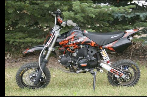
NRG90-F was built for the progressive young rider that is ready for the next level. The throaty 4 stroke power coupled with a 4-spd manual clutch transmission, 36mm front forks, adjustable rear shock, 10 fr / 10 r tires make this a "Pit Bike" in the truest sense. It is a blast to ride and is ready for fun at Home or competition on the track
