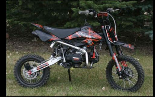
The NRG125-F was designed to be a serious performer. It offers all the features you would expect to find in this class, plus more. A 123cc 4 stroke air / oil cooled engine coupled with a 4-spd moto-x shift pattern manual transmission, inverted front forks, piggy back gas reservoir rear shock, disc brakes and 14 fr / 12 r tires Riding the NRG125-F is addictive!
